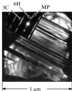
Figure 1. The structure of the heterophase (6H + 3C + MP) SiC crystal.
